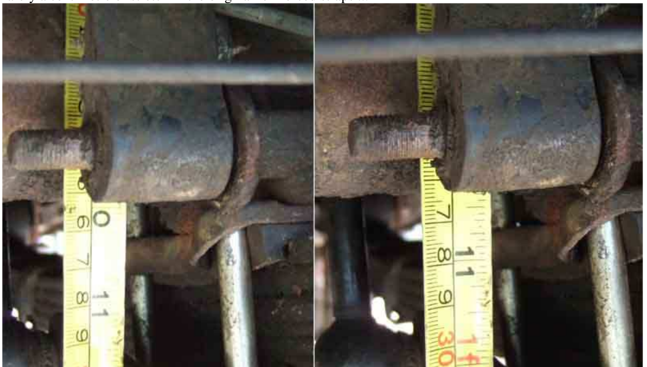
but over 3cm of stretch in the modern 'all rubber'
