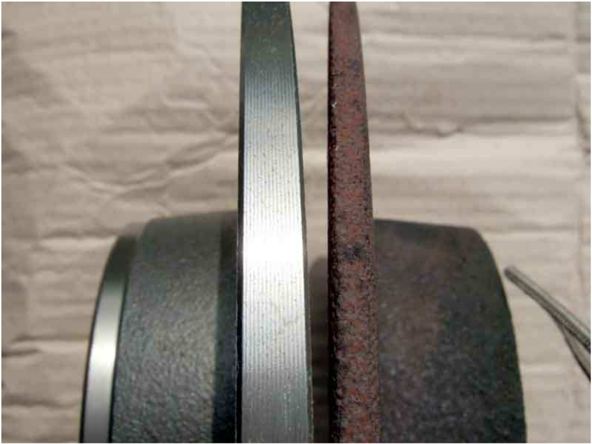
Blued disc. Swept depth also seems to be noticeably smaller than the other disc. This is the very thin disc, but I opt for replacing both.
