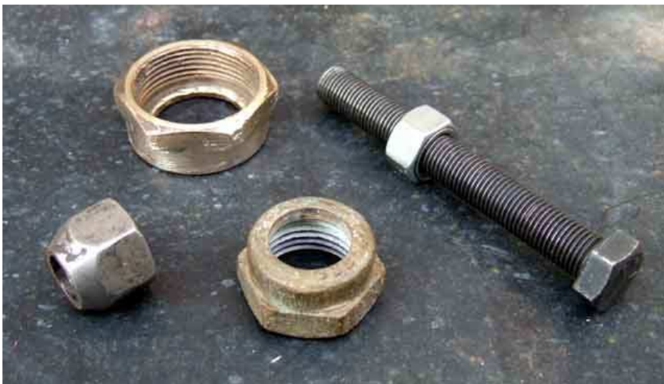
A rear brake cylinder E-clip fitting tool
