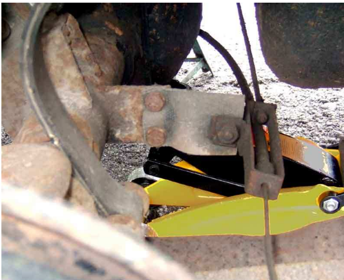
Showing the rear of the diff, where the handbrake pivot used to be, with the anti-roll bar well out of the way.
