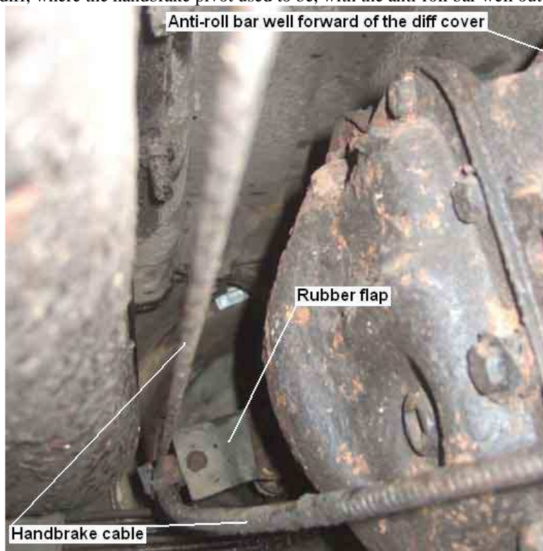
Showing the anti-roll bar, rear pivot on the axle casing, and front pivot mounting point on the body.
