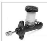
However some suppliers seem to have different versions with a large black cap which fouls the brake master - with the American early i.e. unboosted dual brake masters at any rate. One of these has a plastic reservoir but with the other it is part of the cylinder casting. Moss Europe has three types - the correct early type, specifying GMC1007 for the Mk2 version as well as a cheaper repro. Moss America uses its
