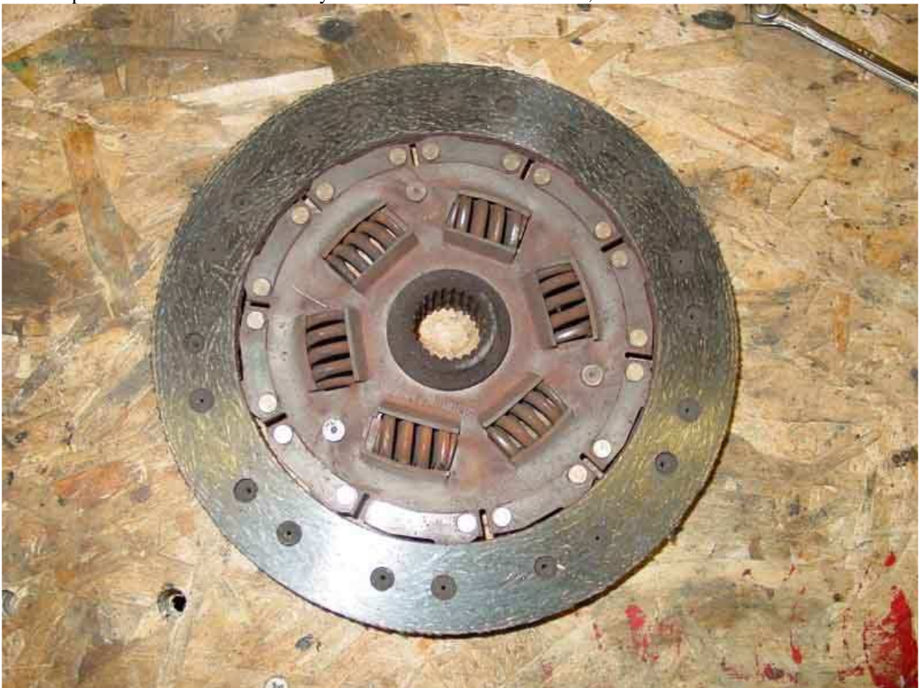
Friction plate with the lands worn away but still well clear of the rivets, not bad for 75k
