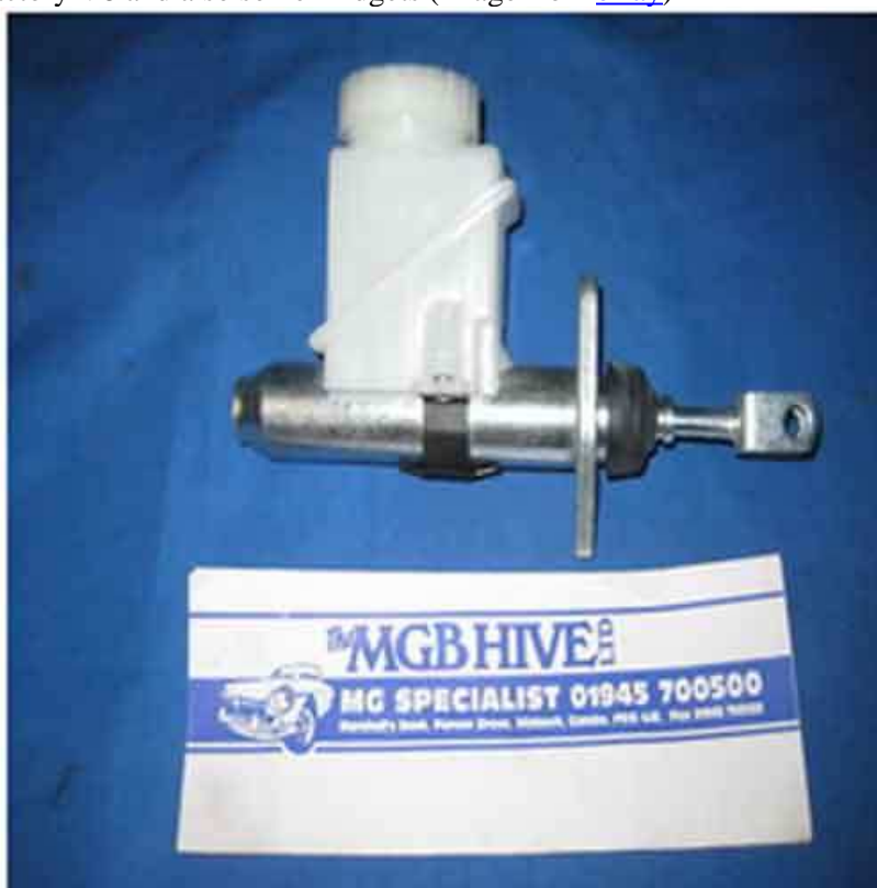
GMC 1011 for the factory V8 and also some Midgets (image from eBay )
