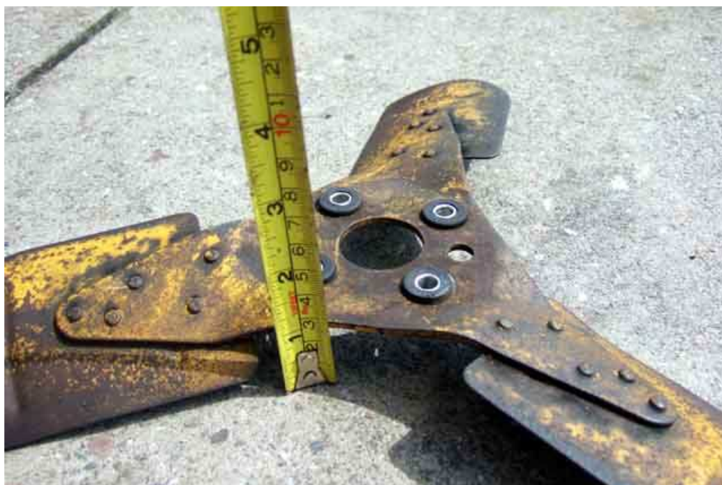
Steve Loft's engine clearly showing the spacer mine lacks, and the blades the correct way round.
