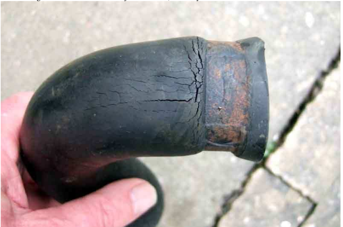
The cracking in Vee's bottom hose after just 15k miles, albeit 7 years...
