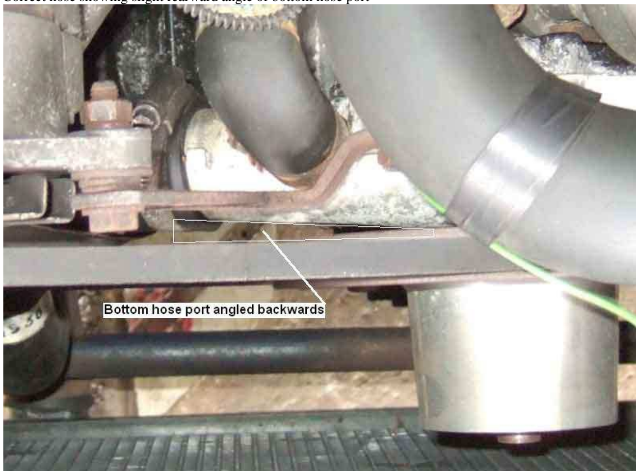
Correct hose showing slight rearward angle of bottom hose port
