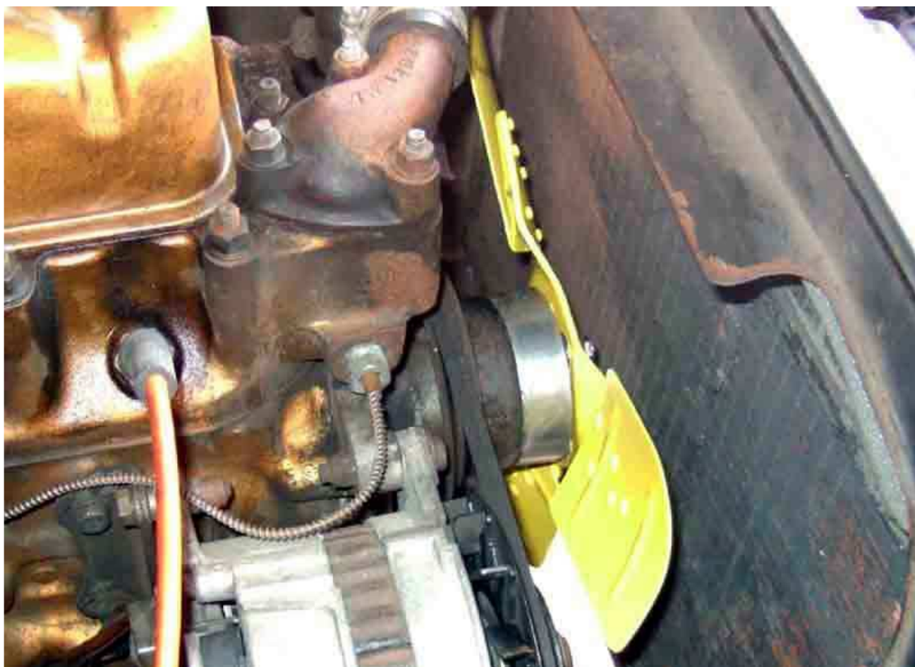
David Bolton's 6-blade fan on a UK 72 shown for comparison. Note the long-nose pump and pulley, and hence no spacer and short bolts (however it could be a short-nosed pump with the spacer inside the deep pulley). Note all these fans rotate clockwise when viewed from the front of the car.
