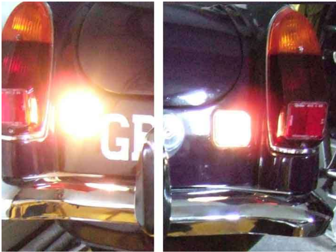
5050-type on the left, 6w festoon on the right - not obviously brighter, just whiter
