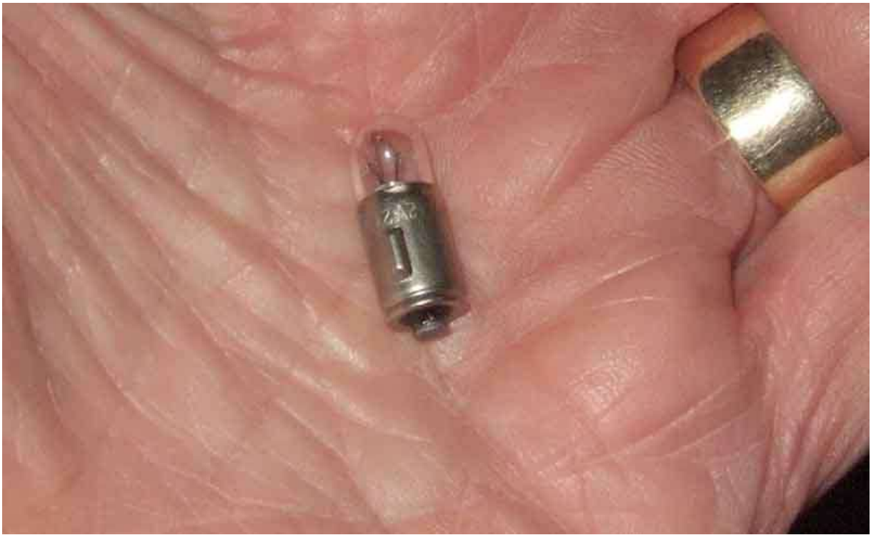
Alternative BA9 (bayonet) fitting (top) to replace tube-type when I was experimenting with LED illumination :
