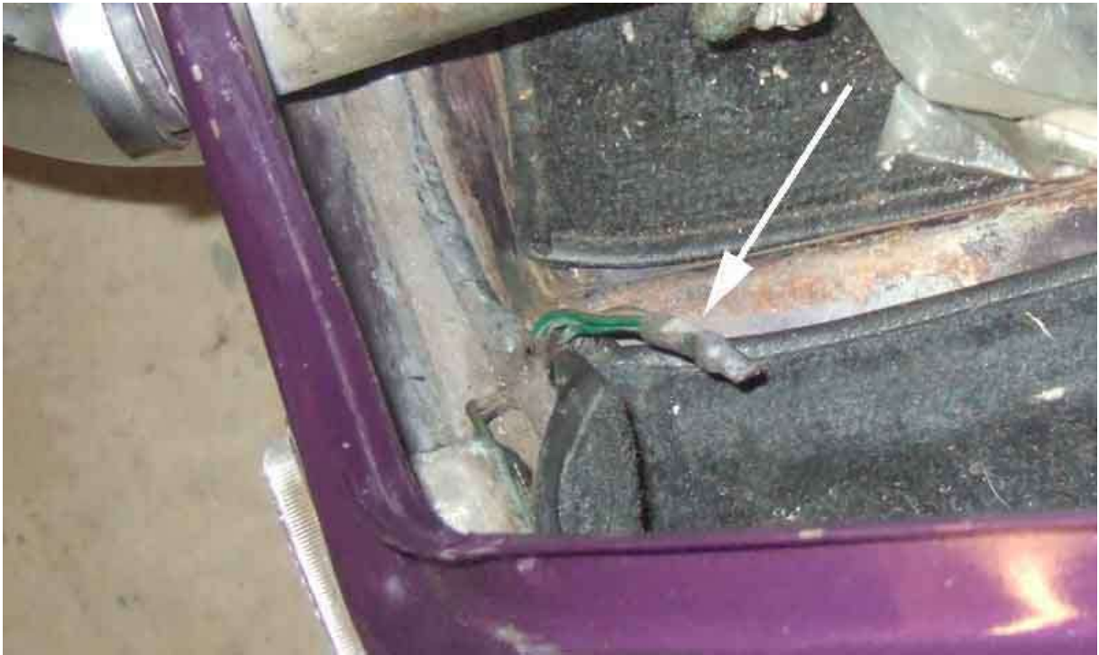
The 2-'pin' (actually two female spades in a three-position holder) arrowed:
