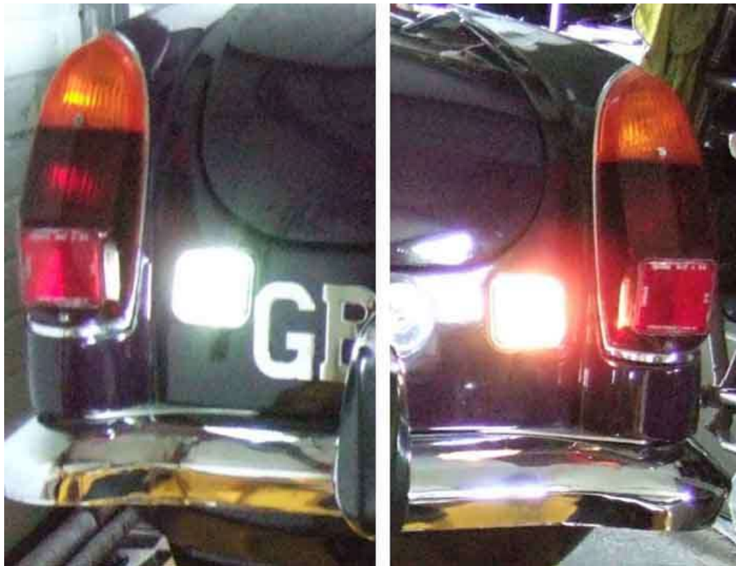
Cree-type on the left - very much brighter than the standard 18w festoon on the right
