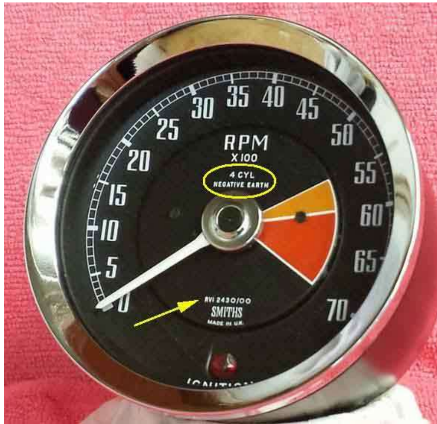
An RVC 2415/00AF (and hence negative earth) as used in markets other than North America, Sweden and Germany from 1973 to the end of chrome bumper production.
