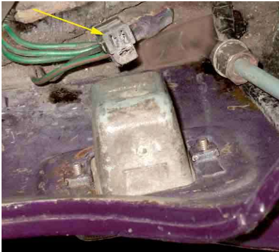
The spades are smaller than the 6.3mm standard at 4.8mm:
