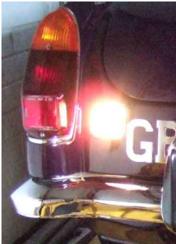
Standard 18w festoon on the left, noticeably brighter than the 6w on the right
