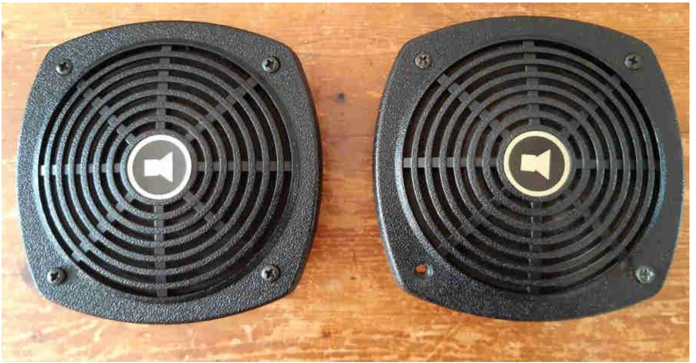
Shrouded to protect the cone and voice-coil from water getting past the drop-glass seals:
