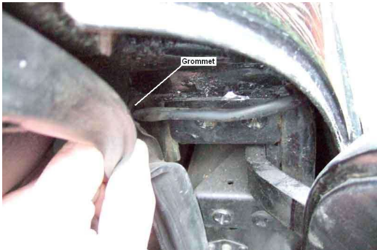
Factory cable routing, showing the grommet in the panel between door space and cabin ...
