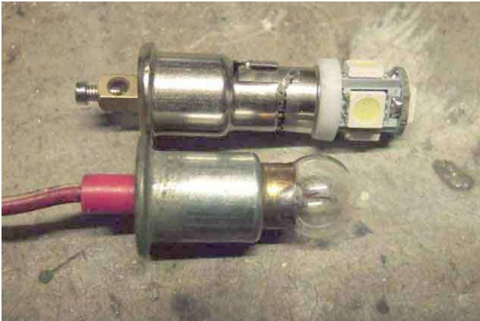
T10 (capless/wedge) holder as received on a replacement harness for a 1980:
