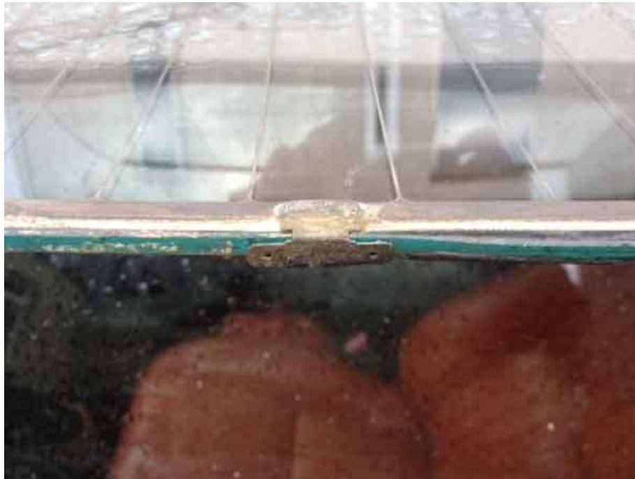
Roy Marshall's replacement glass, showing the very inconvenient connection arrangements.
