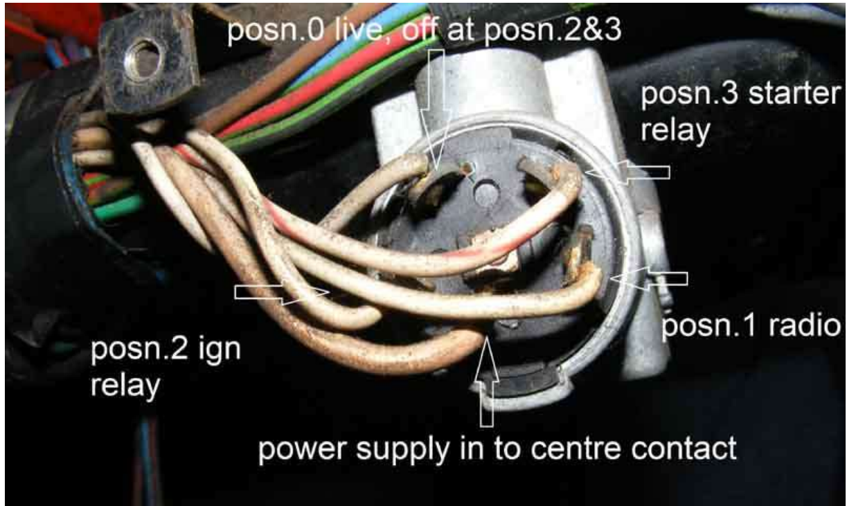
Image from Crispin Allen showing the North American slate/grey anti-runon valve wire at 'posn.0' on a UK 1977:
