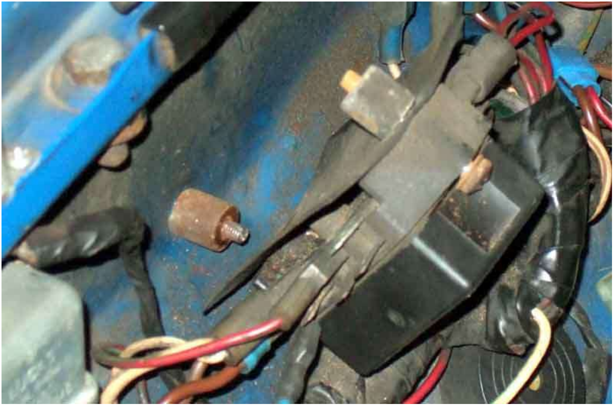
V8 screw is 1 1/2" long, the rusty part is all contained within the nut, it does not protrude beyond it.
