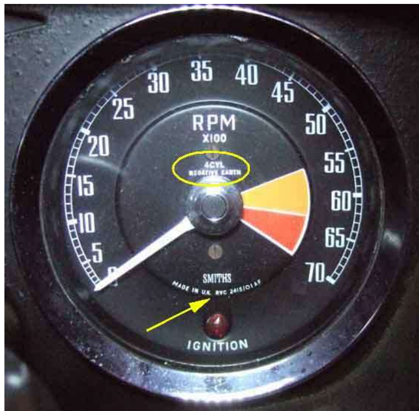
An RVC RVC/1810/00/AF used on V8s, still carrying the polarity indication.
