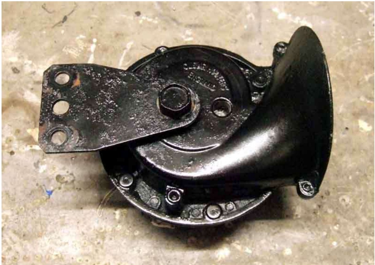
Top of the horn, adjuster screw arrowed
