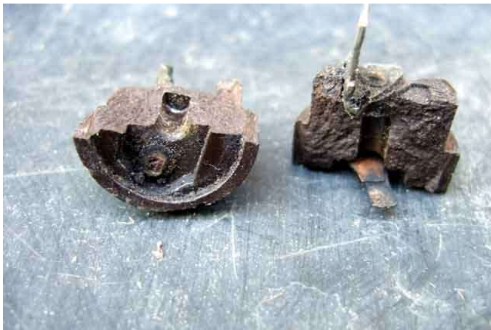
Burnt and pitted contacts, hardly surprising it had failed, surprising it lasted so long!
