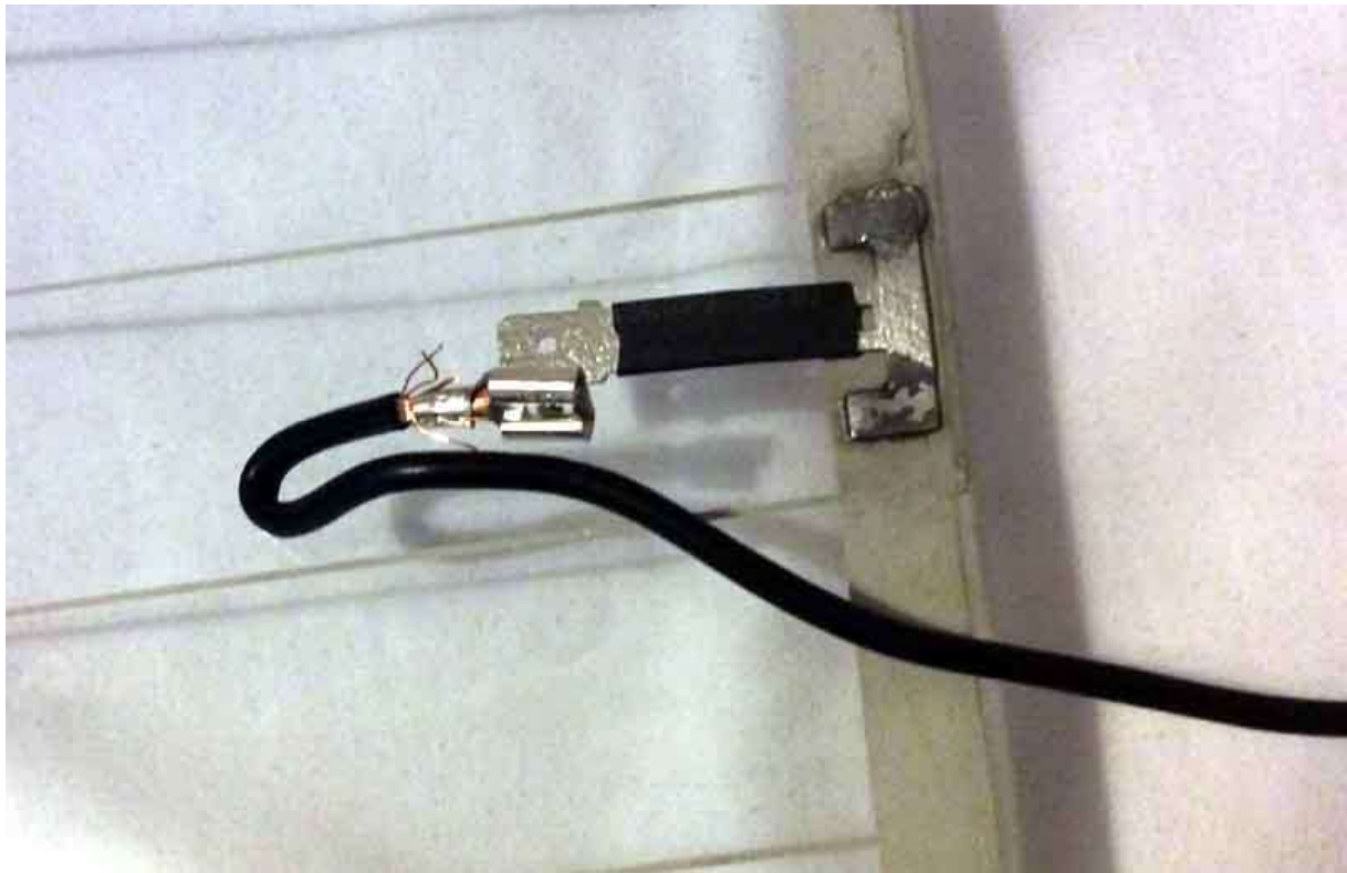
I suggest a right-angle wiring connector is the best way to get a half-way neat installation, however check the size of the spade on your glass first.
