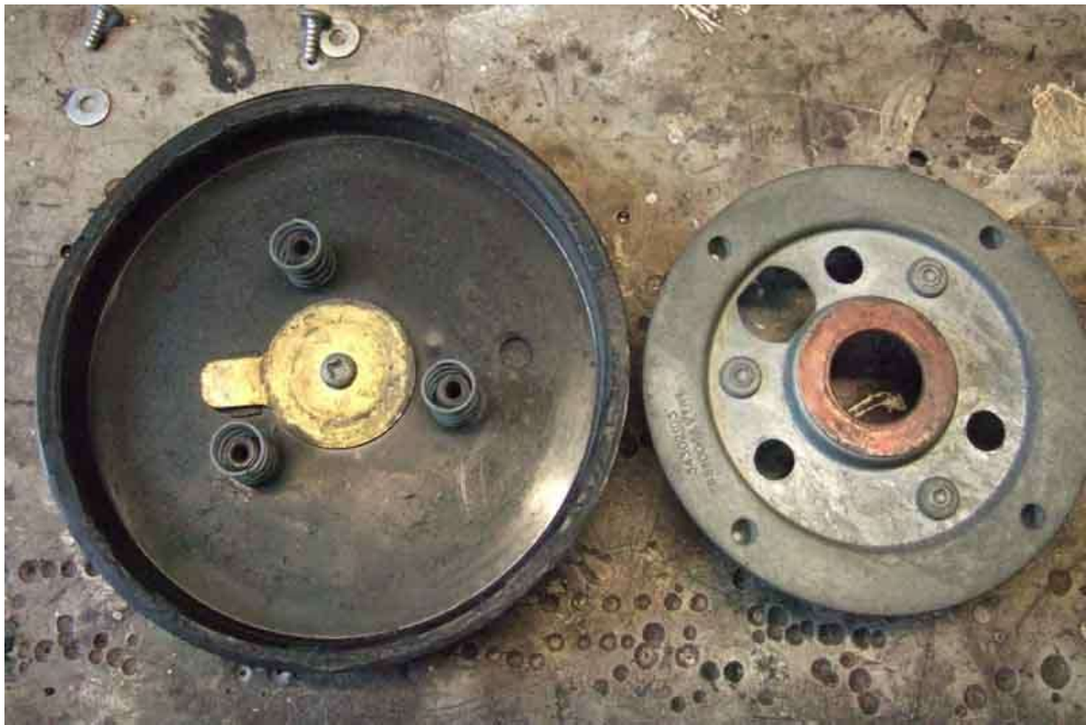
Brass contact on the rubber part and copper on the grey part pretty manky after 45 years:
