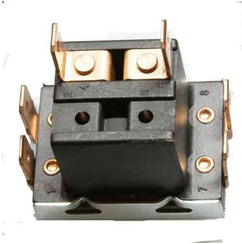
Rocker switch - Blue to 1, Brown to 2, Red/Green to 3:
