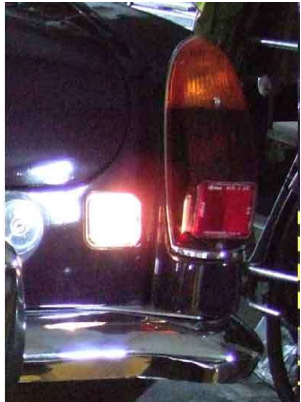
Standard 18w festoon on the left, noticeably brighter than the 6w on the right
