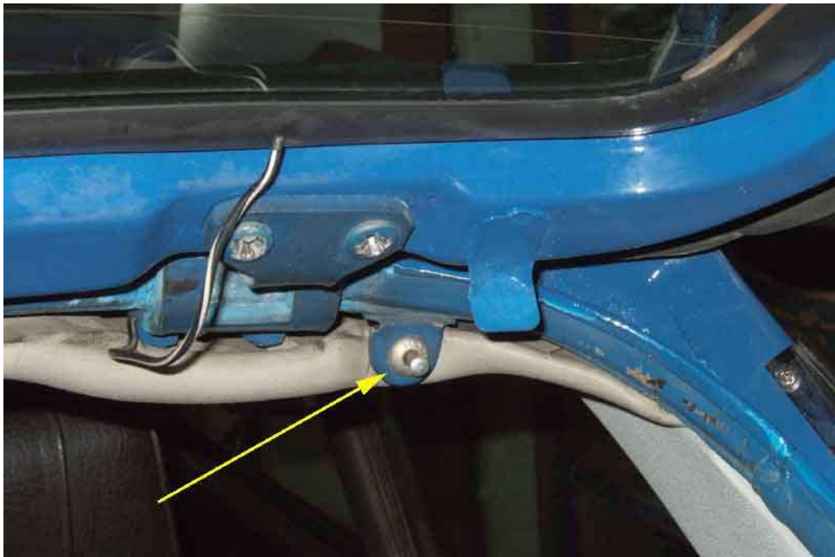
The 12v feeds to the load-space light (purple) and HRW (white/black) come off bullet connections by the right-hand light cluster and go up the C-post.
