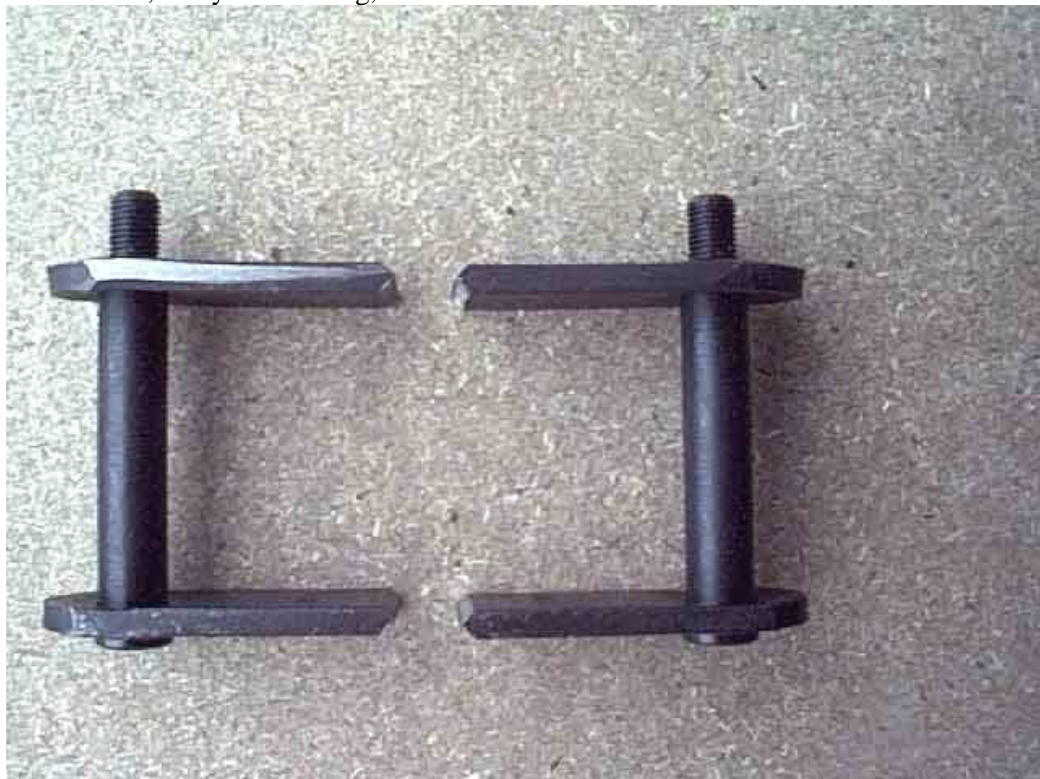
'V' grooves filled with weld then ground flat
