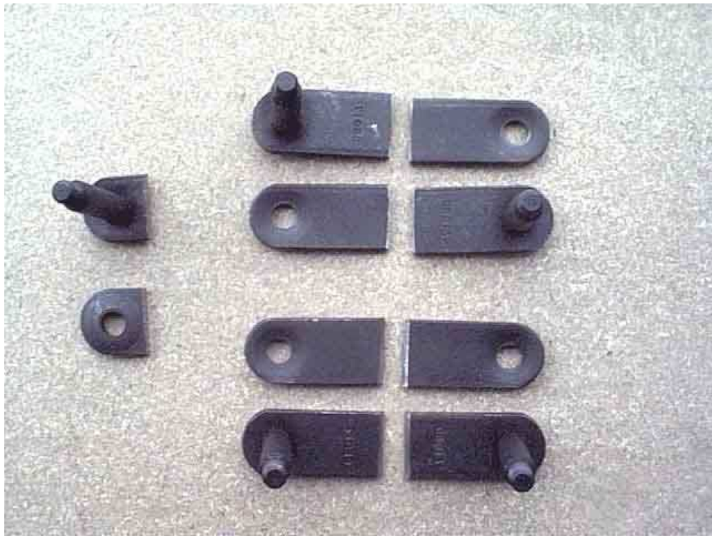
Closing plates attached, ready for welding, ends cut to a 'V'
