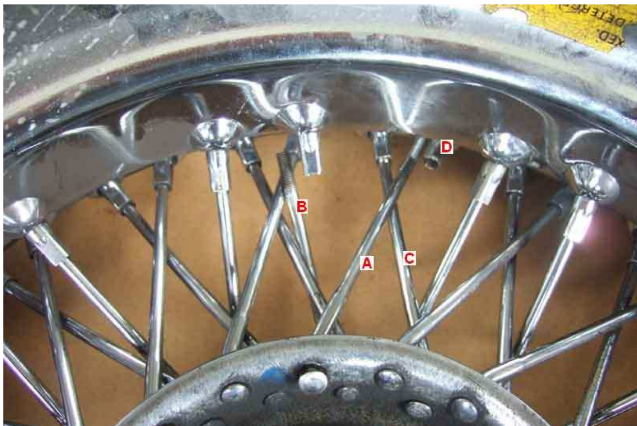
New spoke and long spoke fitted to their nipples prior to tensioning.
