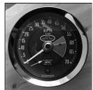
Tachometers were marked with the **original** polarity - positive and negative - from inception, at least until they changed from chrome bezels to plastic for the 1977 model year. But bear in mind that a PO may have changed the internal wiring of a positive earth tach and not changed the legend on the dial.
