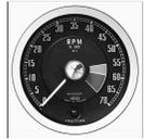
Prior to the electronic tachometer used from October 1964 a mechanical i.e. cable driven from the engine block rev counter was used.
