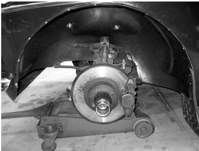
About a week after fitting, I came across an article, on the internet, that had a better way of fitting. Using a piece of edge trim over the wheel arch edge, fit the arch to the inside of the 'guard lip and fasten with screws, through the lip and into the metal of the trim. A much neater looking finish. Ah well, one day I might try it.
