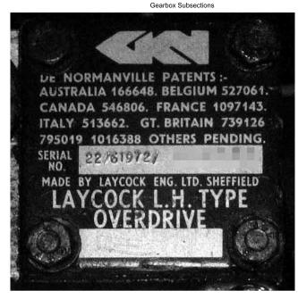
V8s always used a 960tpm speedo drive i.e. for both CB and RB, this is Vee's plate. A number lower than one might expect for a 1975-built car and earlier than Bee's, although V8s probably had their own number series to represent the different operating pressure. Also the earlier 'Laycock/Birfield' plate, so maybe Vee has had a replacement OD ... which may have come from a 4-cylinder!:
