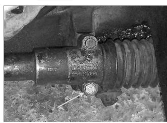
Also noticed that the front rack mounting bolts had been fitted upside down (the rack has to come off to remove the engine as the exhaust manifold that side fouls it), the bolts should be fitted from the bottom as there is a section of weld inside the bracket to hold the bolt while the nut is tightened from above. They had also changed the front bolts, and fitted Nylocs underneath, with lock-washers which is odd.
