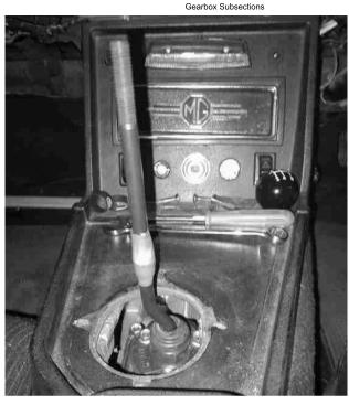
I wrap some cloth round the gear lever, pushing it down through the hole in the centre console, and spread it out to catch metal bits while I shorten the lever with a hack-saw. But first I spin a 3/8" UNC die on to clean up the thread after it has been cut. Thankfully not hardened steel, I cut through in a few minutes.
