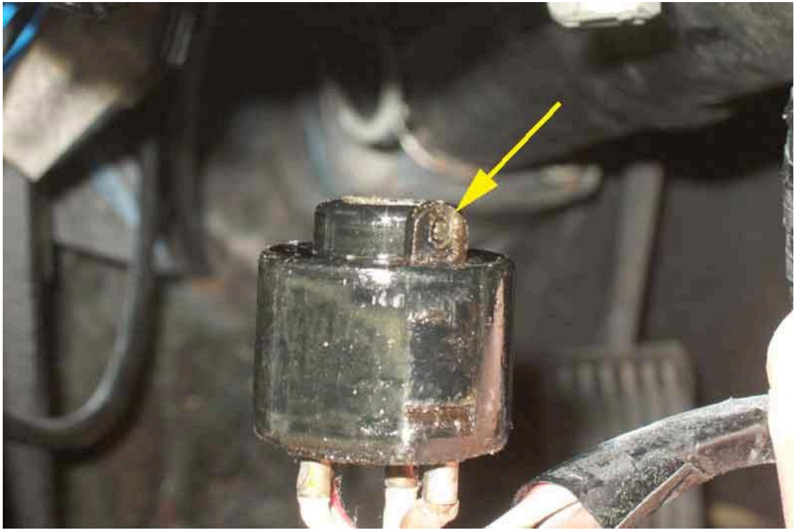
Early LHD side-entry lock - round-head screw facing the driver, although the edges of the socket seem to be peened over into recesses in the switch as well:
