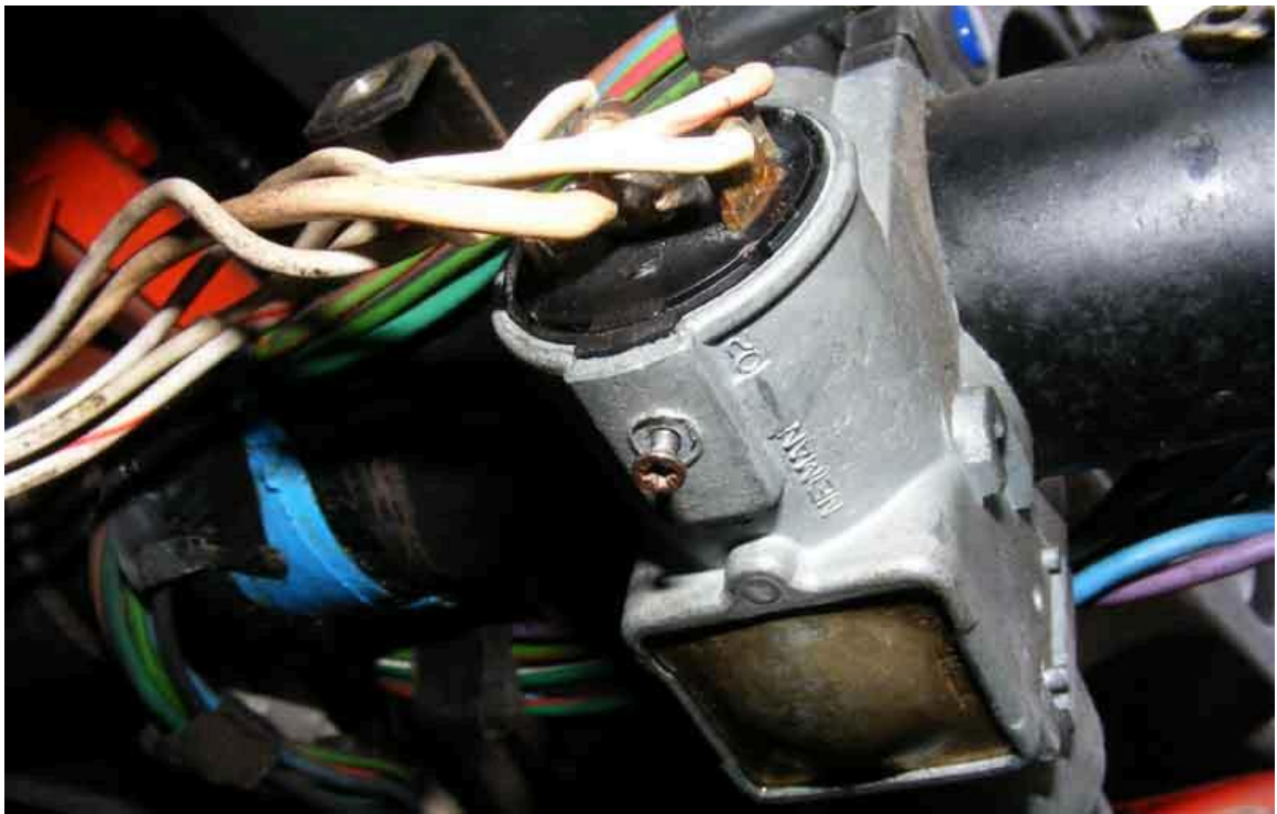
Late UK RB, with a countersunk head screw through the lock body closer to the lock. Both this and the 75 V8 lock above were made by Neiman: ( Crispin Allen )
