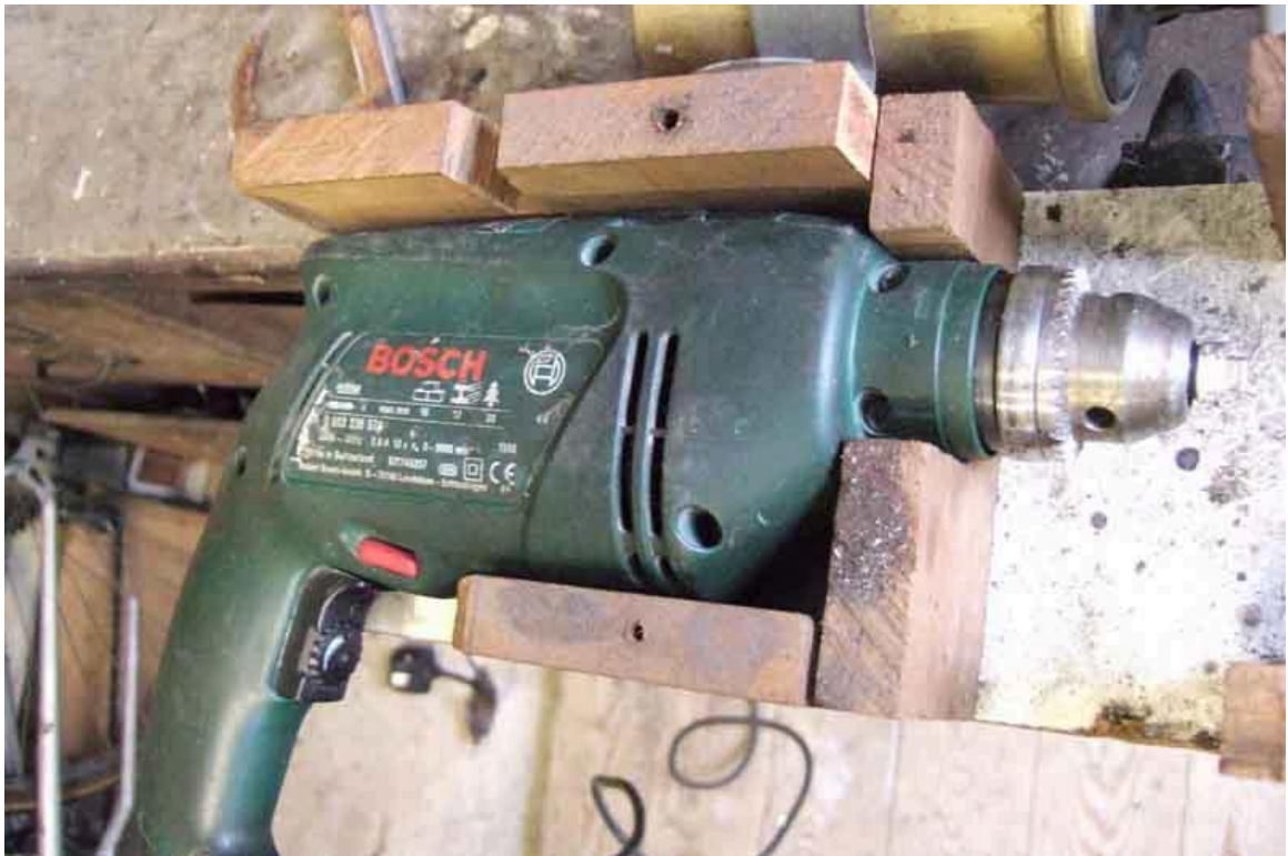
Clamps to hold the drill steady (coil and plugs were so I could drive a strobe light to measure curves)
