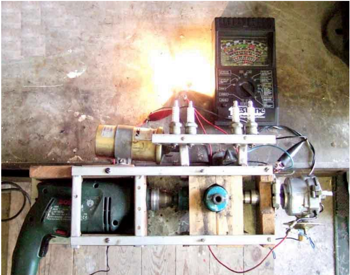
Rig in use to measure dwell on a dwell-meter. The coil and plugs with a degree-wheel fitted to the top of the right-angle drive enable me to plot centrifugal advance curves as well.
