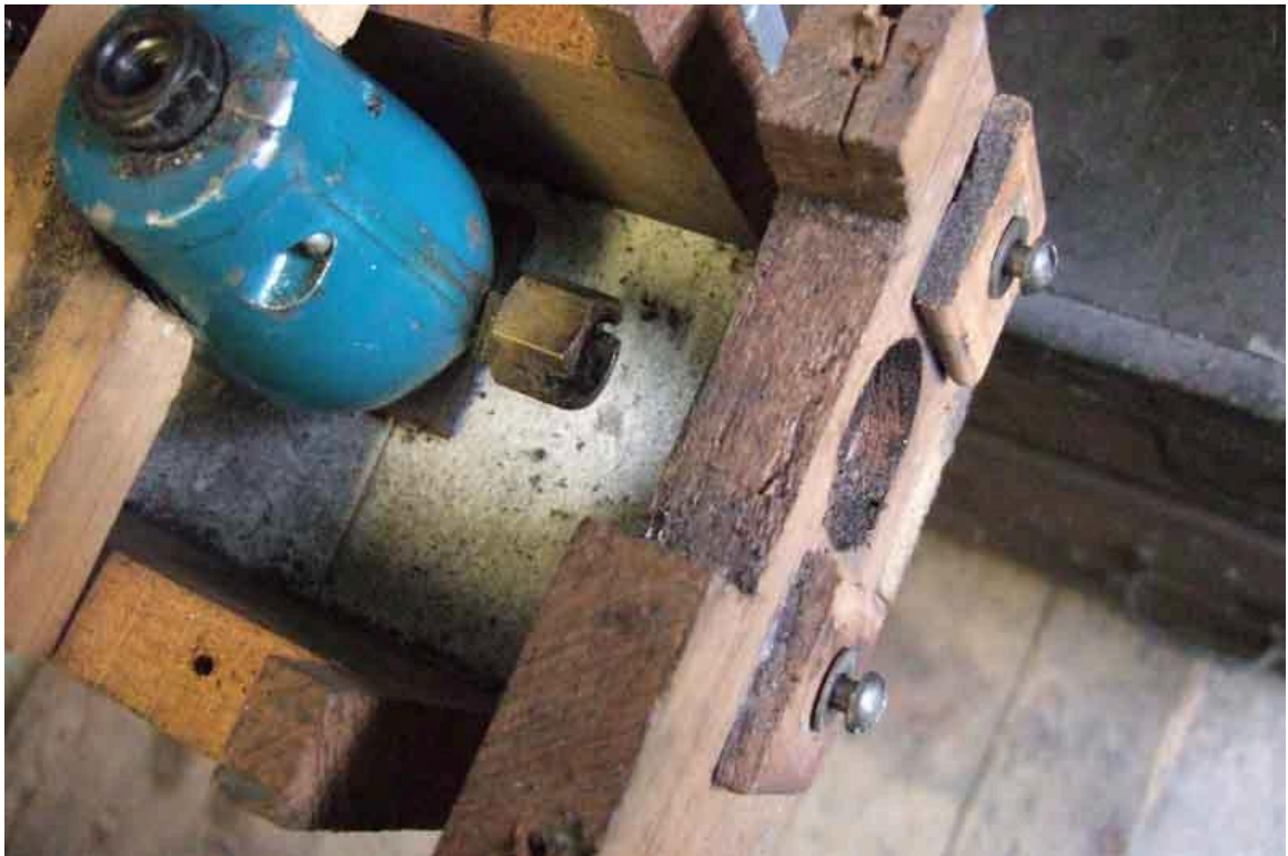
Detail of drive dog, simply a brass plumbing fitting with a slot cut, a bolt through with a nut on the back, ordinarily you would clamp the thread of the bolt in the drill chuck and drive the distributor directly.
